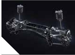
Double ball joints are featured on each of the two upper and two lower control arms, allowing for control of the smallest movements from driver inputs and the road surface. This arrangement helps optimise the suspension geometry and create more precise steering response with better initial effort. Contributing to the LC's weight-saving programme, the upper control arms are made of lightweight forged aluminium.
