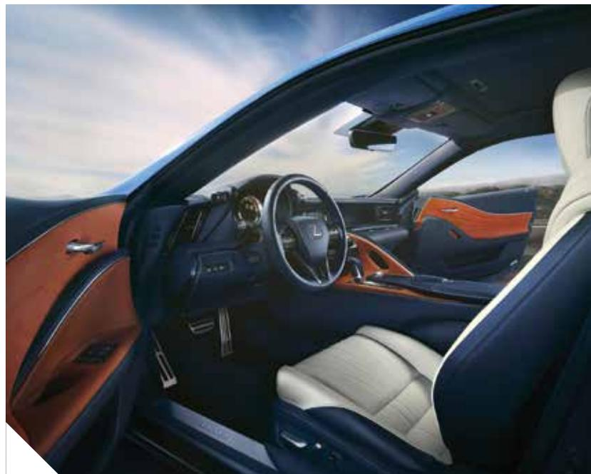
The information displays are arranged in order of importance, with the most critical positioned closest to the driver's sightline, within the dashboard's upper display zone. All are positioned at the same height, to reduce the degree of eye movement required for the driver to read them. The instrument binnacle houses the latest development of the TFT (thin film transistor) metre technology introduced in the Lexus LFA supercar, including a moving central ring.
