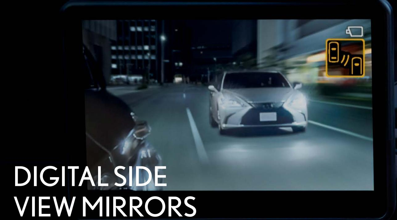
The new Lexus ES sedan was the first production vehicle to be fitted with digital side mirrors. Japanese market models are available with small cameras positioned on the front doors, which feed real-time images to five-inch monitors located inside the cabin, at the base of the front pillars. The cameras are designed to operate consistently in all weather conditions, and will automatically enhance the images shown when the turn signals are activated.
