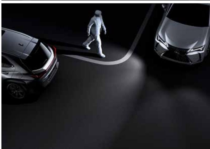
The Pre-Collision System (PCS) couples with Dynamic Radar Cruise Control. The system can operate relative to a vehicle ahead that is traveling 10 to 180 km/h (7 to 110 mph). Dynamic Radar Cruise Control with Road Sign Assist (RSA) can quickly reset the vehicle speed setting in accordance with the speed limit information recognized by RSA.
