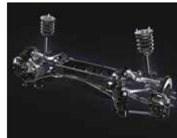
Double ball joints are featured on each of the two upper and two lower control arms, allowing for control of the smallest movements from driver inputs and the road surface. This arrangement helps optimise the suspension geometry and create more precise steering response with better initial effort. The upper control arms are made of lightweight forged aluminium, contributing to the LC's weight-saving programme.
