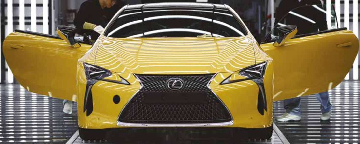
The new production line at Motomachi has a pure white finish from floor to ceiling to create an environment that helps the team members focus on their work. Each person will spend as much as 20 minutes working on every car, combining hand and eye skills with the use of tablet devices to check and re-check the quality of each process. Skills – both mental and technical – are constantly developed to support a “no compromise” mindset when it comes to achieving Lexus’ rigorous quality standards.
