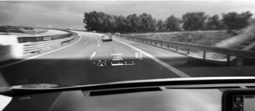
THE HEAD-UP DISPLAY SYSTEM ALLOWS THE DRIVER TO CONCENTRATE ON THE ROAD AHEAD WITH MINIMAL DISTRACTION.
